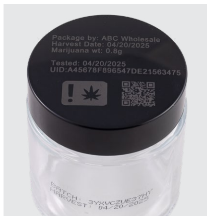
Laser on plastic cap of a glass jar
