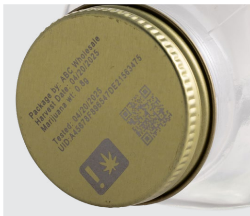
Laser on a metal cap of a glass container
